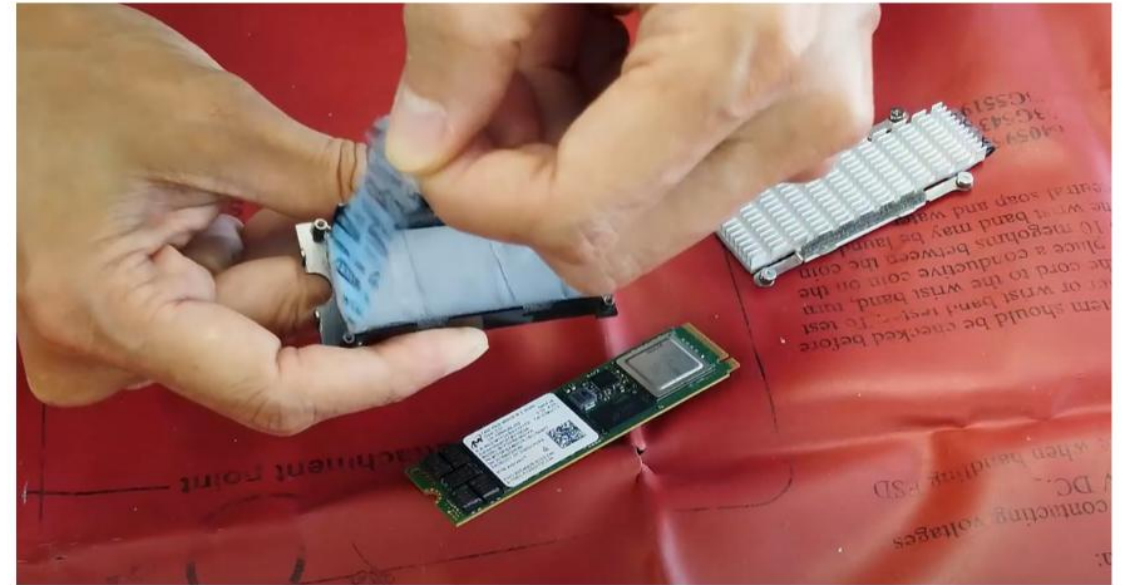
Apply a new thermal pad to the replacement M.2 adapter
