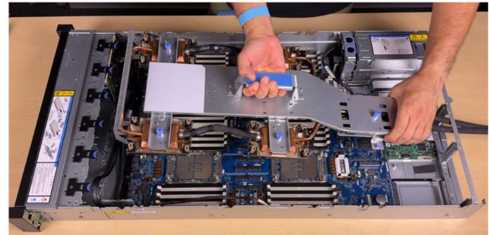
Installing the Neptune core module to the system with the shipping bracket
