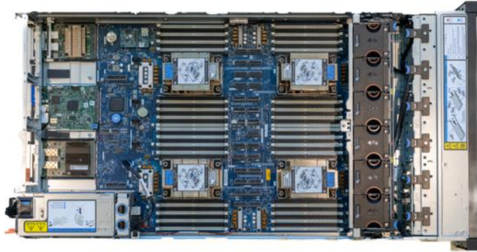
Air-cooling system without air baffle
