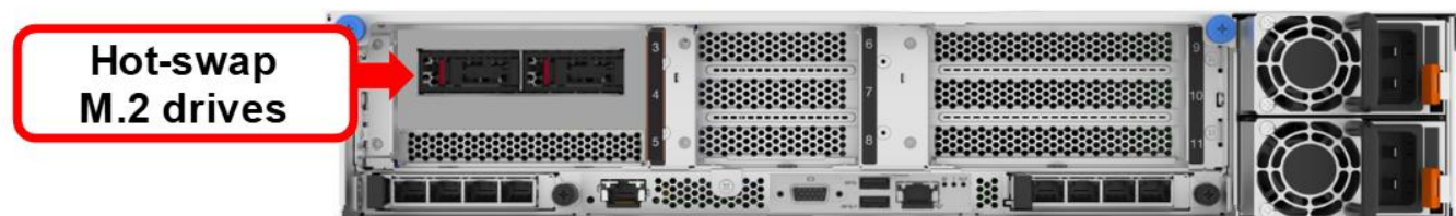
Three-riser configuration with optional hot-swap M.2 drives
