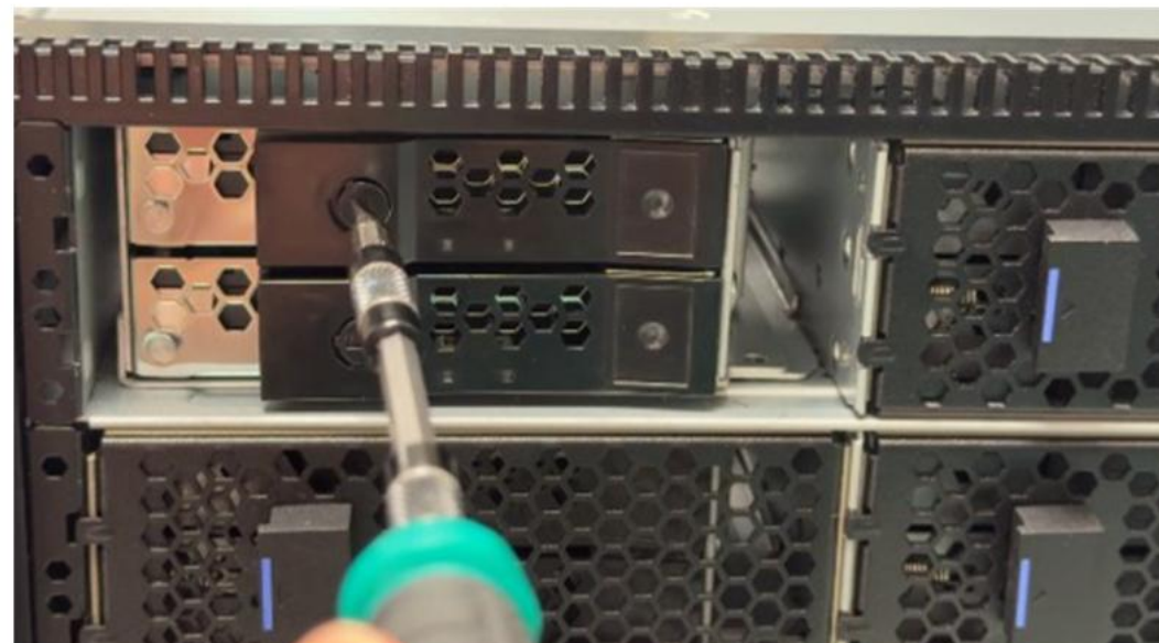
Unlock the CXL memory module handle
