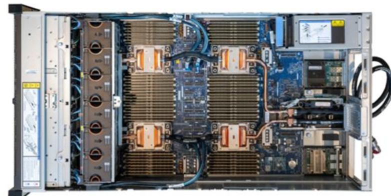
System with processor liquid-cooling Neptune core module installed
