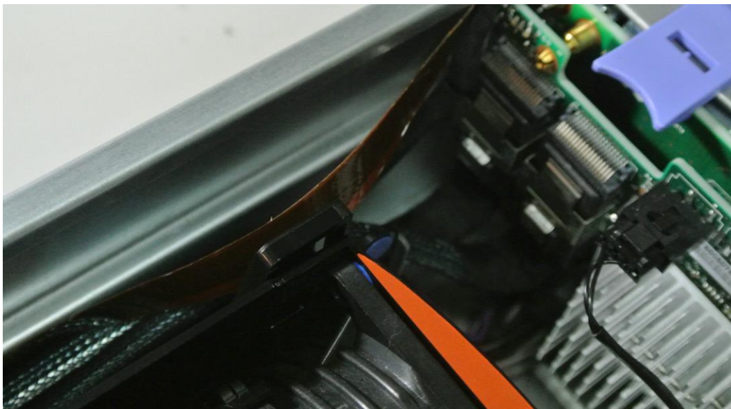
Figure 47: Flat Cable Connecting the Front KVM Panel to the System Board
