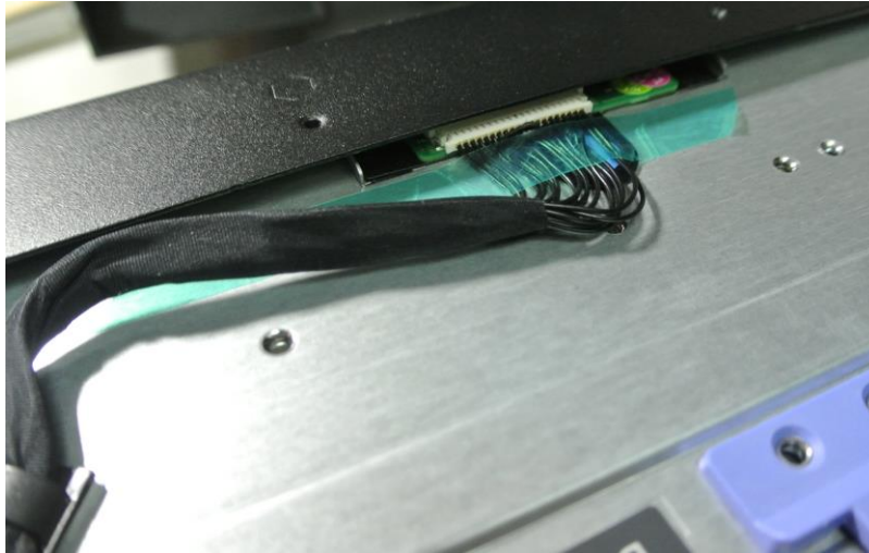
Figure 49: Cable Connected to the Operator Panel
