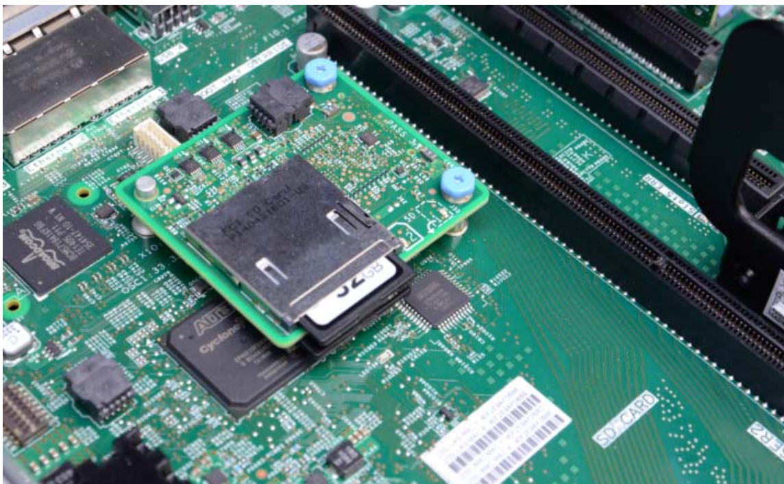
Figure 30: SD media adapter installed in the x3650 M5
