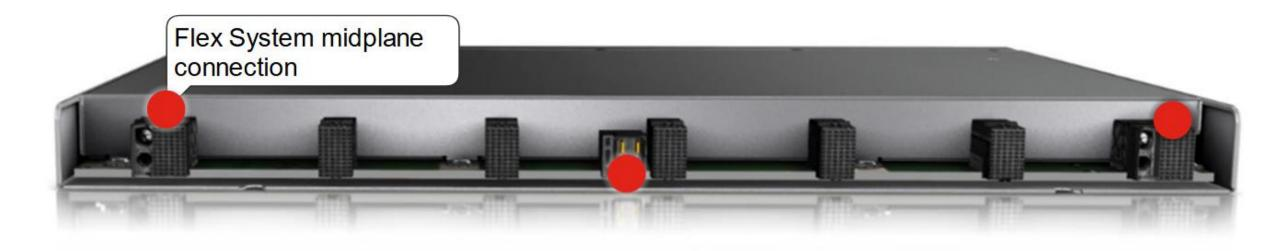
Connections at the rear of the NE2552E Flex Switch provides twenty-eight internal ports that can be configured as twenty-eight 10 GbE ports, twenty-eight 25 GbE ports, fourteen 50 GbE ports, or certain combinations of 10 GbE, 25 GbE, and 50 GbE ports.
