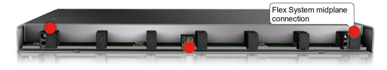
Connections at the rear of the NE2552E Flex Switch provides twenty-eight internal ports that can be configured as twenty-eight 10 GbE ports, twenty-eight 25 GbE ports, fourteen 50 GbE ports, or certain combinations of 10 GbE, 25 GbE, and 50 GbE ports.
