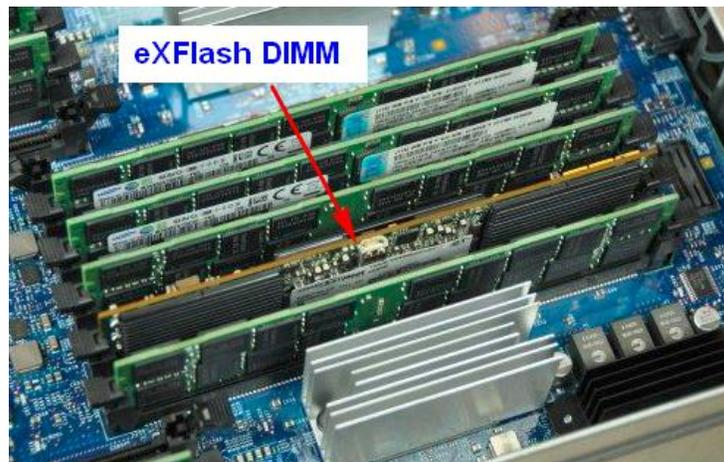
**Figure 3: Lenovo eXFlash DIMM installed in the memory slot with RDIMMs**
