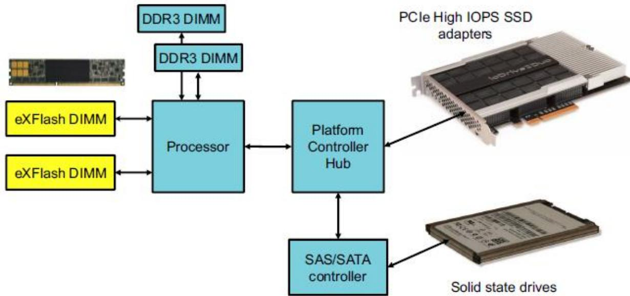
**Figure 2: Lenovo eXFlash DIMMs placement**
