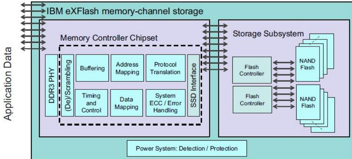
Figure 11: eXFlash DIMM block diagram
