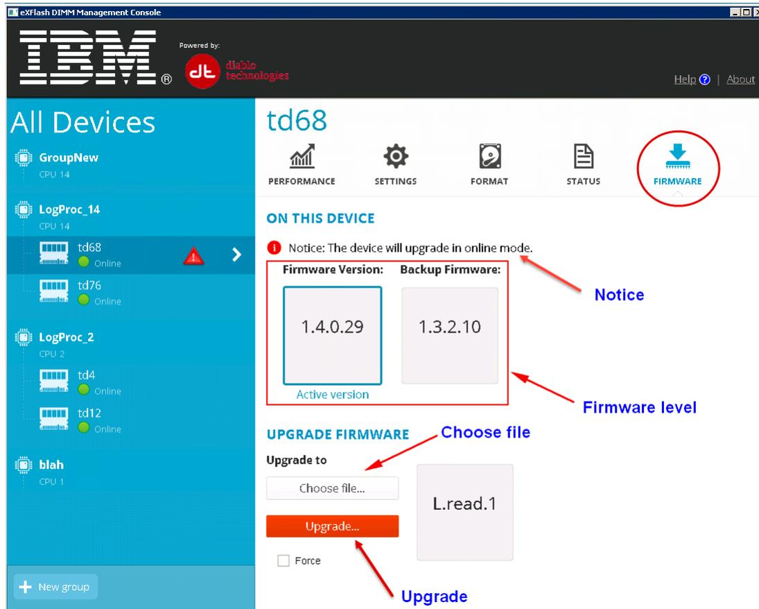
**Figure 5: eXFlash DIMM firmware upgrade using the management console**
