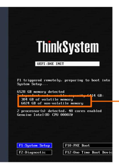
In this example, the DCPMMs are provisioned with App Direct mode, so the entire DCPMM capacity (6024 GB) is non-volatile memory. The 384 GB of volatile memory is supplied by the DRAM DIMMs.
