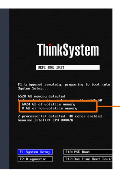
In this example, the DCPMMs are provisioned with Memory mode, so the DCPMM and DRAM DIMM capacity is volatile memory. There is no non-volatile memory available on the system.
