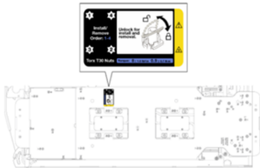
Figure 238. Screw tightening/loosening sequence on the shipping bracket label
