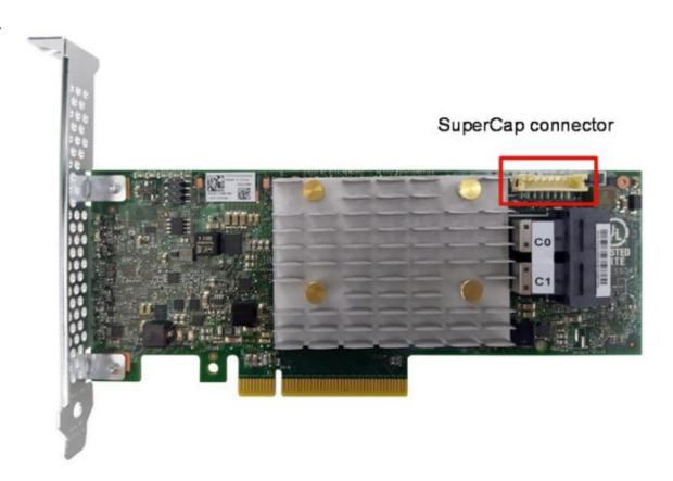
**Note**: The RAID 9350-8i adapter looks very similar to the 4350-8i HBA and RAID 5350-8i adapter, but it has a SuperCap connector on the PCB.
