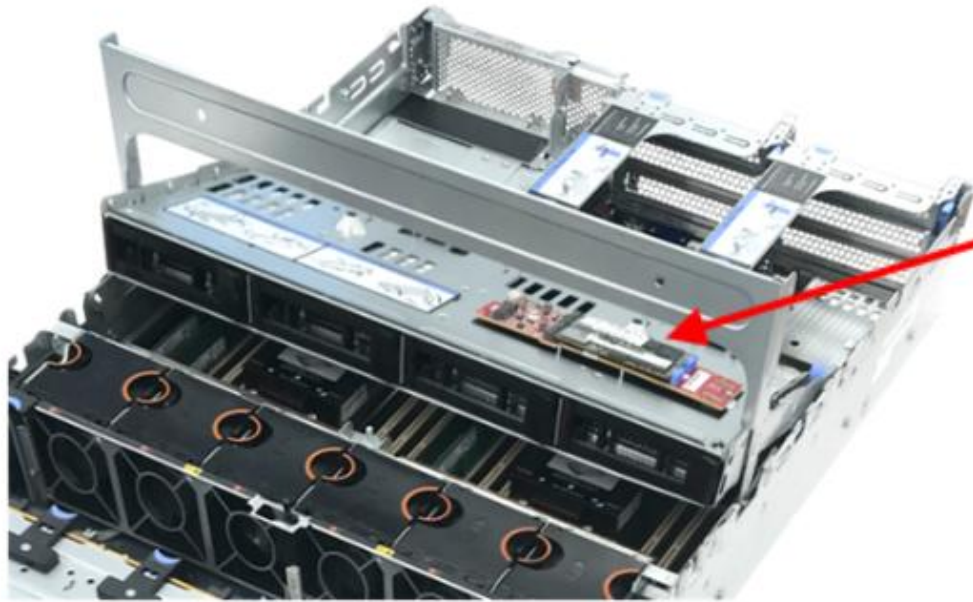
Four 3.5-inch mid-chassis hot-swap drive bays
