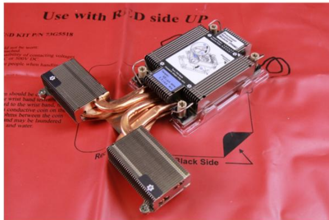
Performance heat sink For processors with a TDP of more than 250 watts
