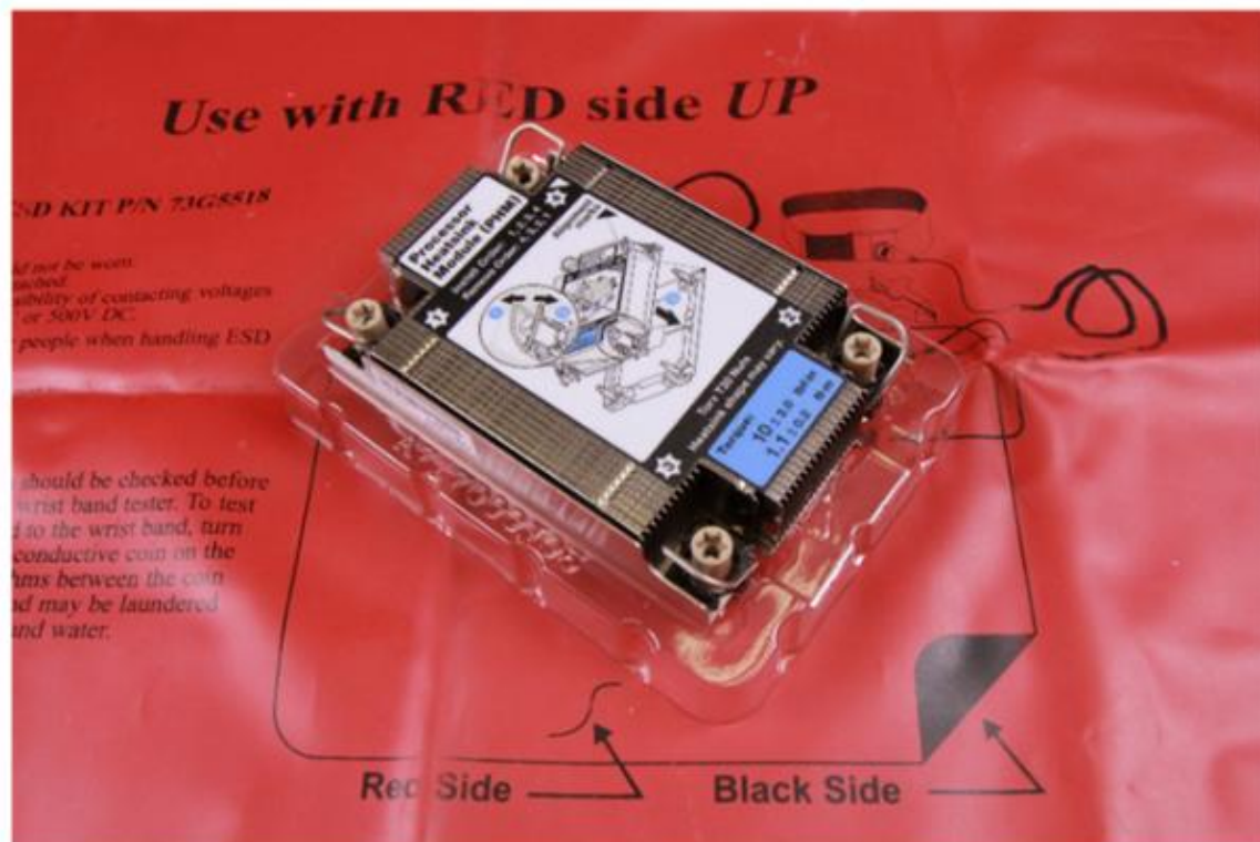
Standard heat sink For processors with a TDP of less than 205 watts
