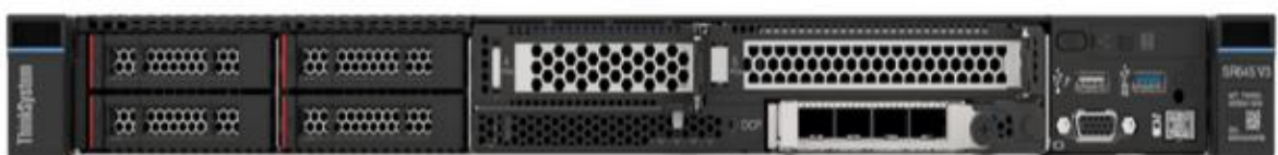
Four 2.5-inch drives, two PCIe 5.0 slots, and one OCP slot
