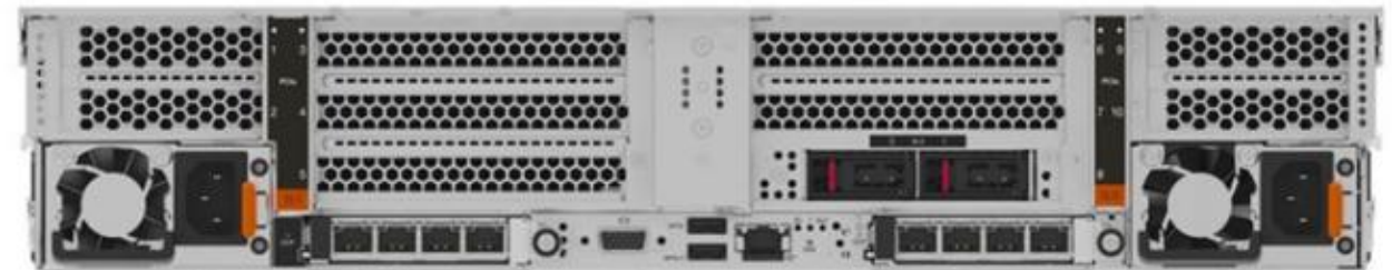
Rear hot-swap M.2 in slot 8 (can also be used with rear 2.5-inch or 3.5-inch drive bays)
