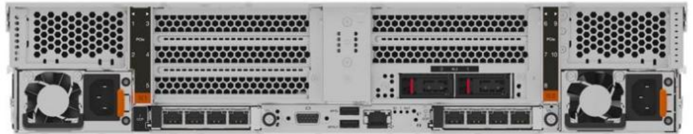
Five PCIe slots and two hot-swap M.2 drives
