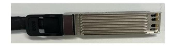
Finned connector for the switch side
