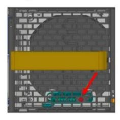
Power (rear) side inlet to connector side outlet – indicated by blue dots on the power inlet side.
