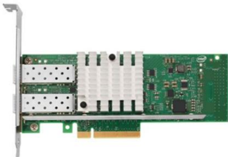
Intel X520 dual-port 10 GbE SFP+ adapter
