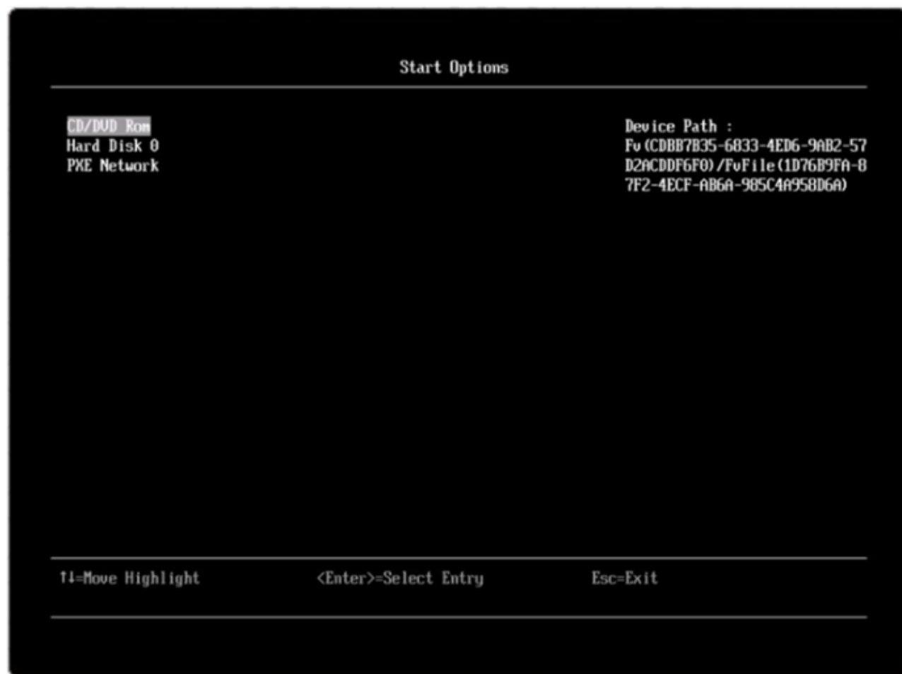
Boot order in UEFI setup screen
