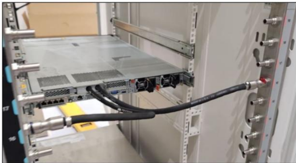
ThinkSystem SR630 V3 with a water-cooling module installed in a rack
