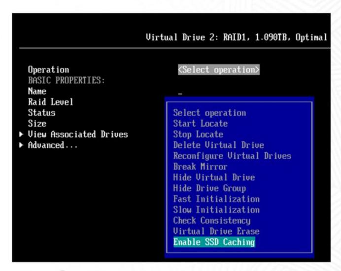
Virtual Drive 2: RAID1, 1.090TB, Optimal <Enable SSD Caching> Operation BASIC PROPERTIES: Name Raid Level <RAID1> Status  $\langle 0ptimal \rangle$ 1.090 TB Size ▶ View Associated Drives ▶ Advanced...
