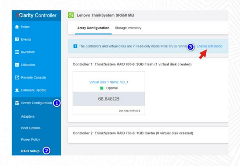
Log in to the LXCC Web UI and select Server Configuration → RAID Setup → Enable edit mode.
