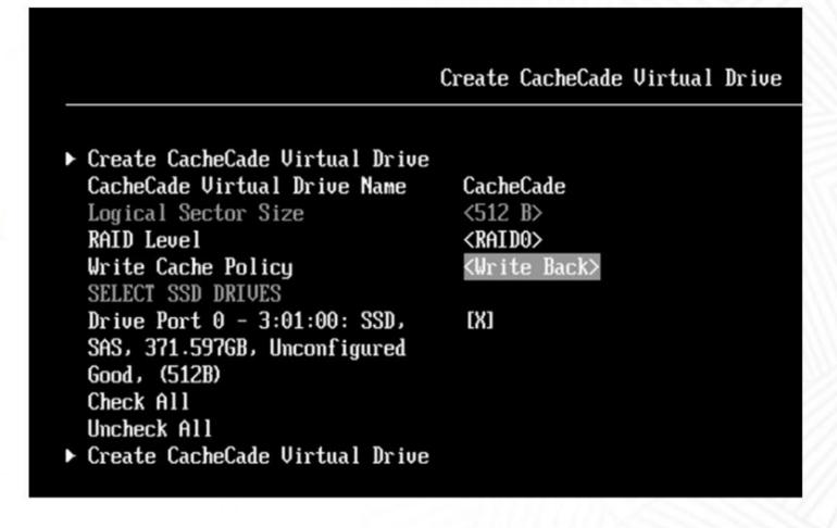
Enable the SSD caching on any of the existing Virtual drives by selecting the VD that you want to enable SSD caching on under the Virtual Drive Management menu.
