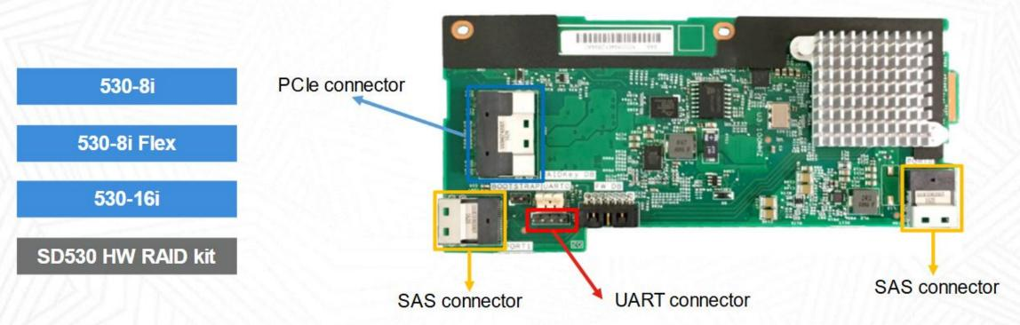
Note: The UART connector debug port requires a special cable and Broadcom support to gather detailed IOC status.
