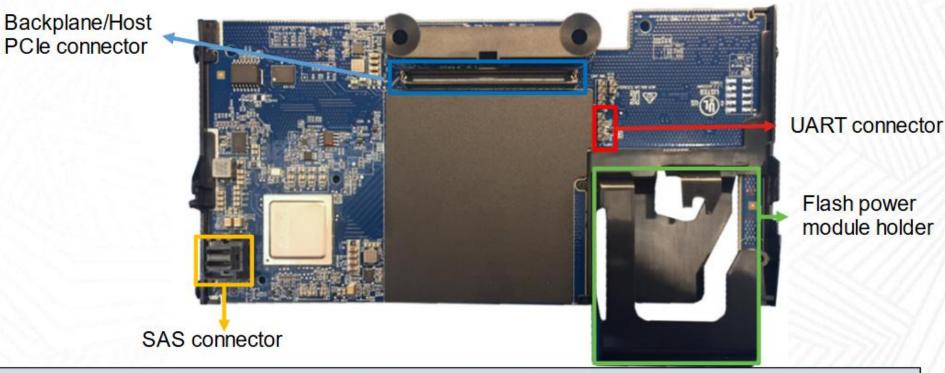
Note: The UART connector debug port requires a special cable and Broadcom support to gather detailed IOC status.
