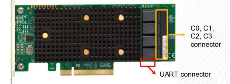
Note: The UART connector debug port requires a special cable and Broadcom support to gather detailed IOC status.
