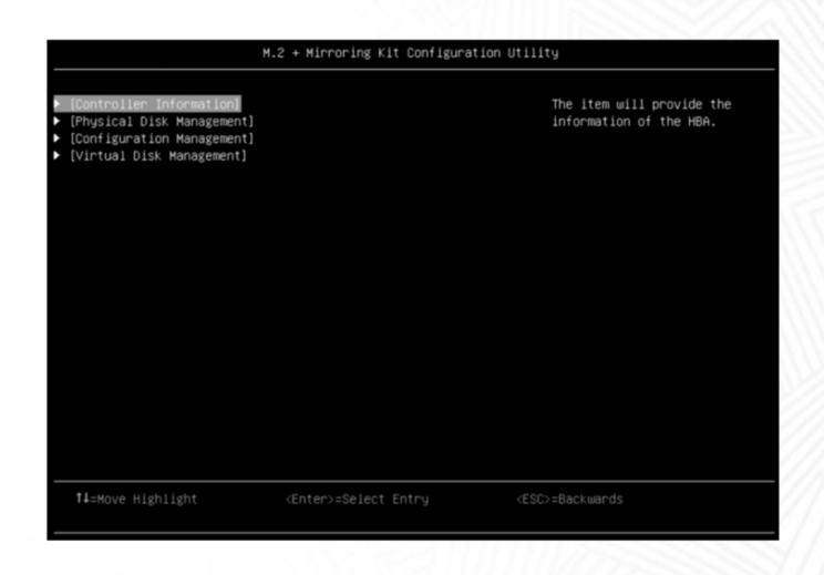
The Dual M.2 boot adapter includes an UEFI driver that provides controller and drive inventory/configuration function in the HII Configuration Utility. Inventory only in LXCC Web UI.
