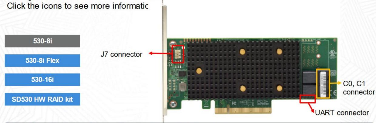
Note: 1. The J7 connector is the only difference between the 530-8i and 430-8i adapter.
