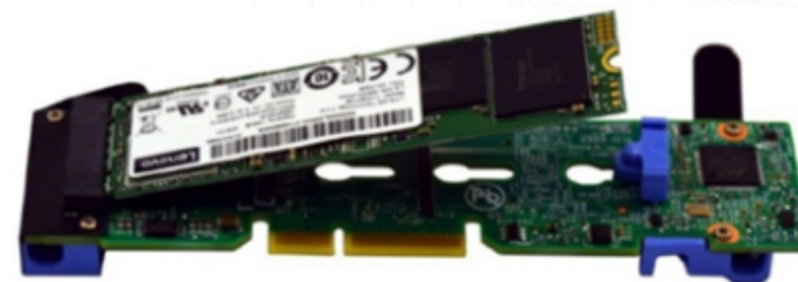
Dual M.2 boot adapter with one 128 GB M.2 drive partially installed (second M.2 drive is installed on other side of adapter).
