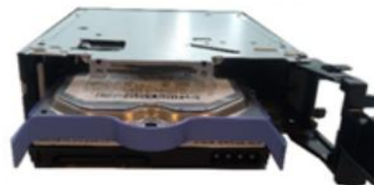
3.5-inch SSD to 5.25-inch tray convertor kit (rear view with tray open)
