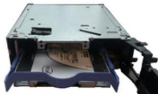
2.5-inch SSD to 5.25-inch tray convertor kit (rear view with tray open)
