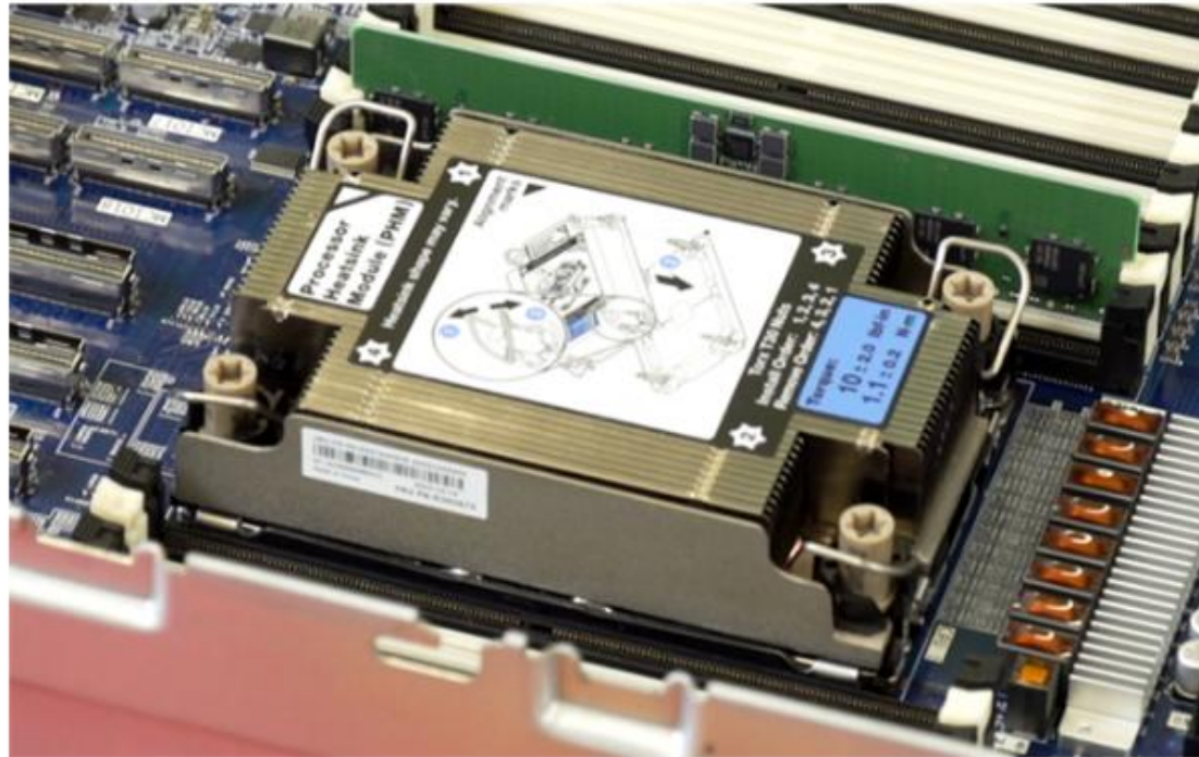
A 1U standard heat sink in an SR850 V3
