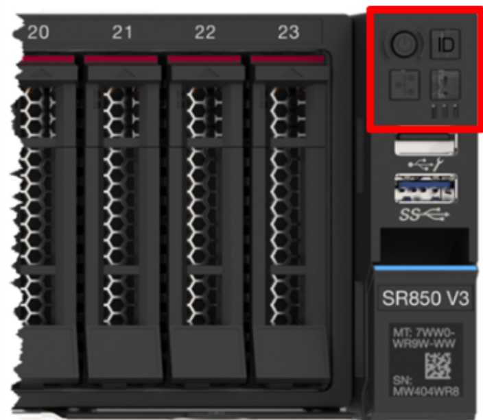
Front diagnostic LED panel on an SR850 V3
