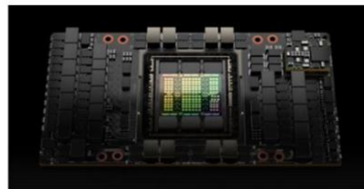
An NVIDIA H100 GPU without a heat sink
