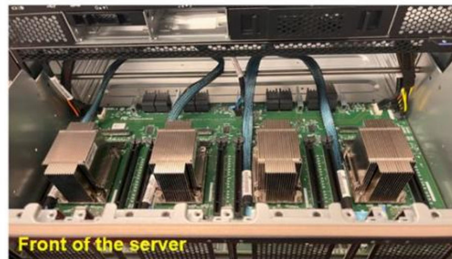
A switch board without PCIe adapters installed
