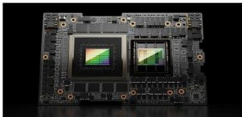
An NVIDIA H200 GPU without a heat sink
