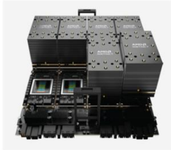
An AMD GPU board with eight MI300X GPUs
