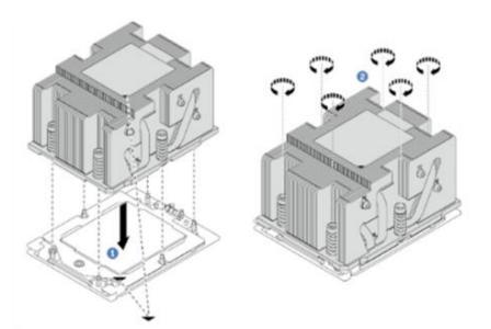
Installing a performance heat sink
