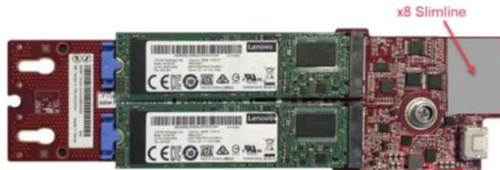
M.2 SATA/NVMe drive PCIe 4.0 backplane (new for the ThinkSystem V3 series)
