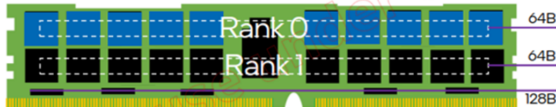
Dual Rank MRDIMM – Two ranks operate simultaneously to combine data lines
