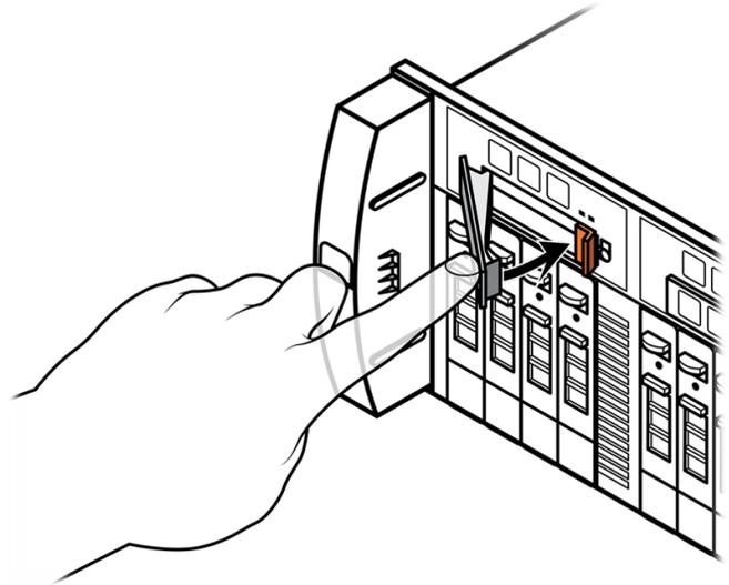
**Figure 8-9. Latching the Replacement NVRAM Module**
