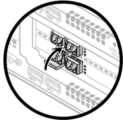
**Figure 14-16. Installing Optical Transceivers and Connecting Cables**
