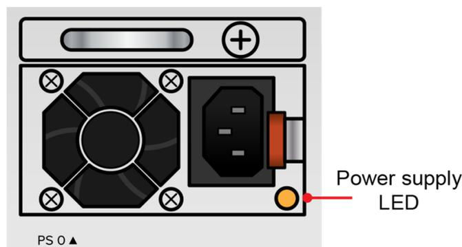
**Figure 3-3. Power Supply LED – Faulty**
