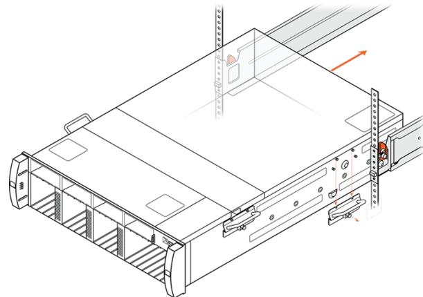
**Figure 11-14. Installing the Replacement Chassis, Part 1**
