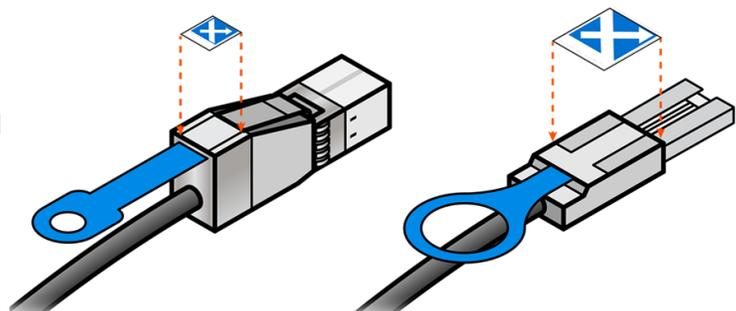
Figure 5-7. Labeling the Replacement Cable
