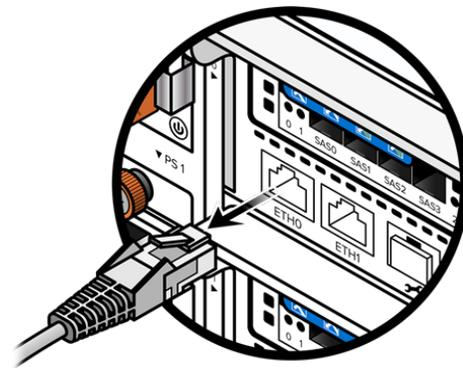
Figure 11-6. Disconnecting a Management Cable
