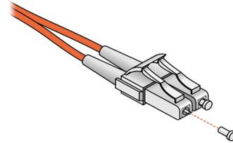
**Figure 7-6. Protecting Optical Cable Tips**
