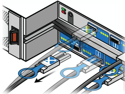
Figure 5-5. Removing a SAS Cable (Storage Shelf)
