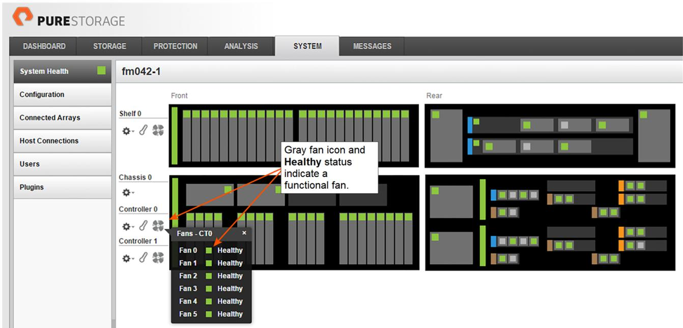
**Figure 10-14. GUI Indication of an Operational Fan**
