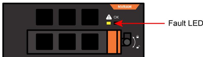
Figure 8-4. Faulty NVRAM Module LED Indicator
