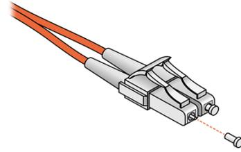
Figure 11-5. Protecting Optical Cable Tips
