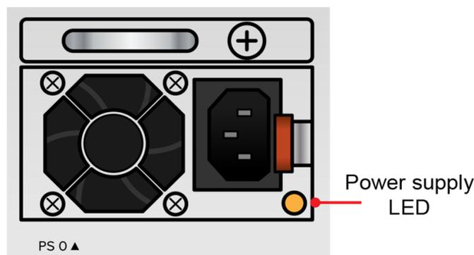
**Figure 4-3. Power Supply LED – Faulty**
