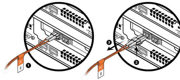
Figure 10-4. Disconnecting a Host Cable (Fibre Channel Shown)
