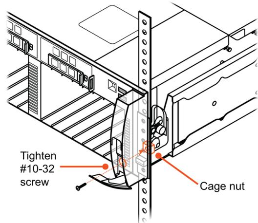
**Figure 11-16. Securing the Chassis to the Front of the Rack**
