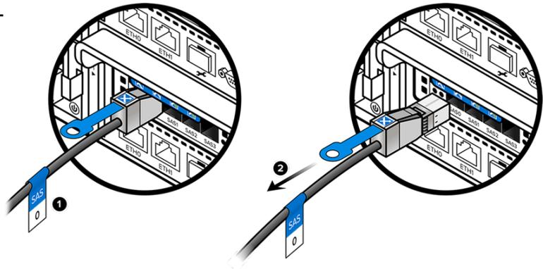
**Figure 11-2. Disconnecting SAS Cables**
