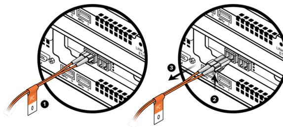
Figure 13-5. Disconnecting a Host Cable (Fibre Channel Shown)
