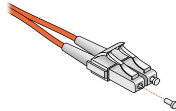
**Figure 10-5. Protecting Optical Cable Tips**
