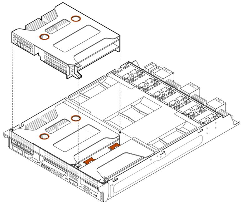
Figure 13-16. Install New Riser 0
