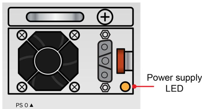
**Figure 2-3. Power Supply LED – Faulty**
