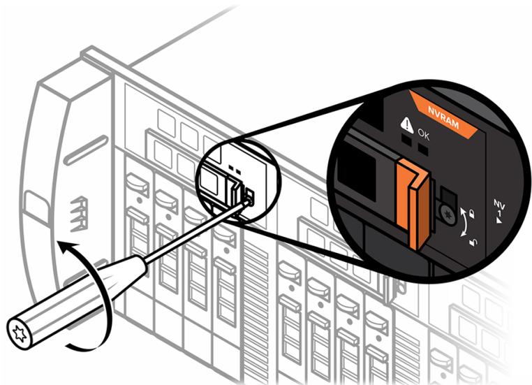
**Figure 8-10. Tightening the NVRAM Module Lock**
