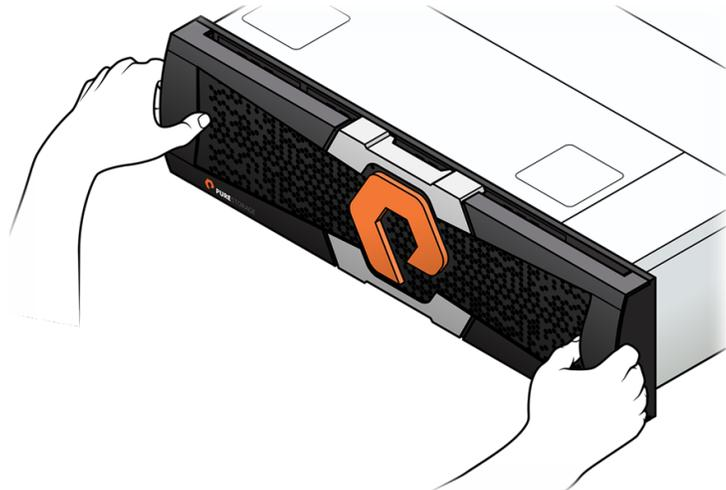
Figure 8-1. Removing the Bezel
