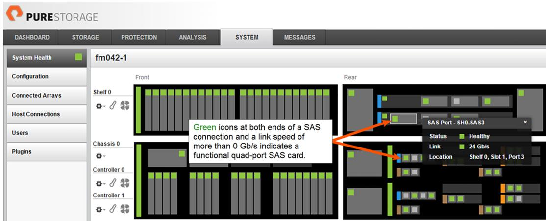
**Figure 13-22. GUI Display Showing a Healthy Quad-Port SAS Card**
