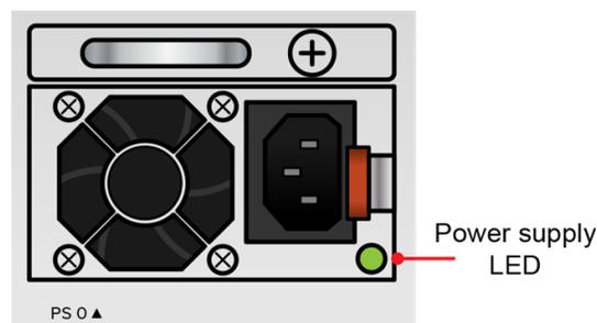
Figure 1-10. Power Supply LED – OK
