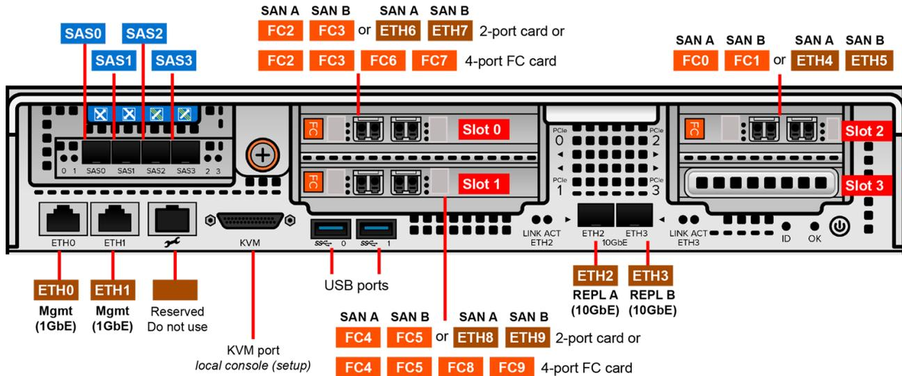
Figure 13-4. FlashArray//M Controller Ports (2-Port PCIe Cards Shown)
