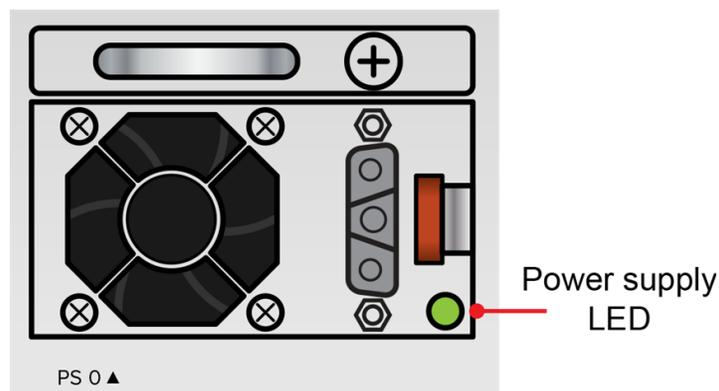
Figure 2-10. Power Supply LED – OK
