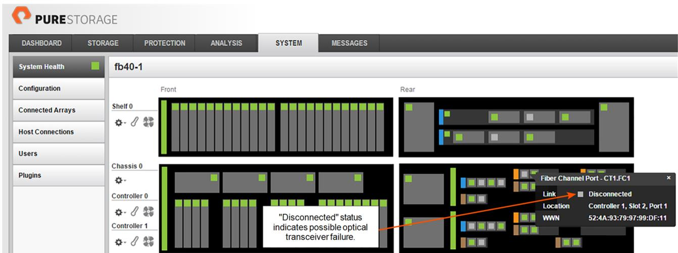
Figure 6-1. GUI Indication of Possible Optical Transceiver Failure
