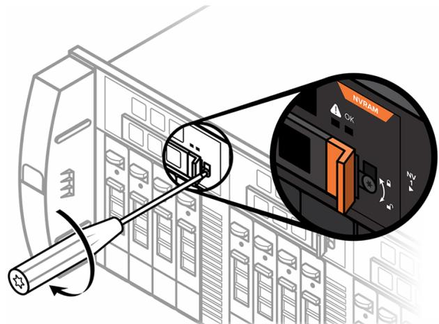
Figure 8-5. Unlocking the NVRAM Module
