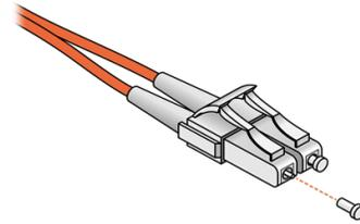
Figure 6-4. Protecting Optical Cable Tips
