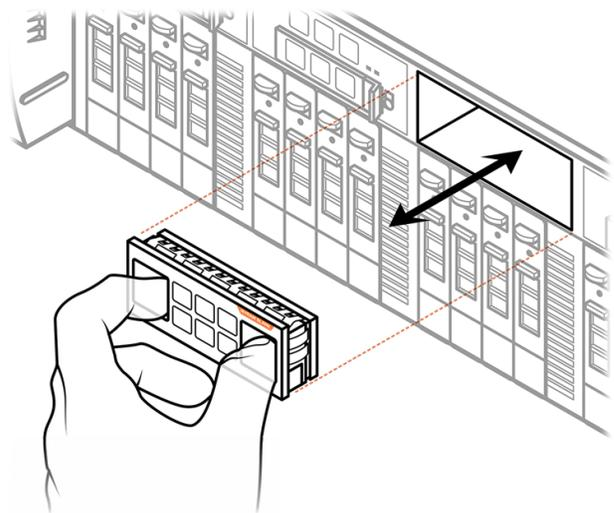
**Figure 9-1. Installing an NVRAM Blank**
