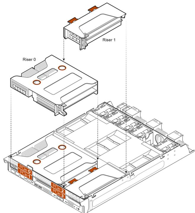
Figure 14-15. Reinstalling the Risers
