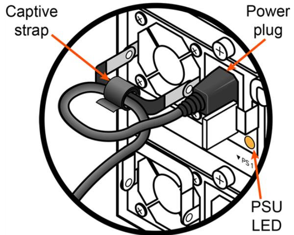
**Figure 17-5. Securing the Power Cord**
