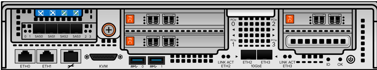
**Figure 14-1. FlashArray//M Controller Panel**
