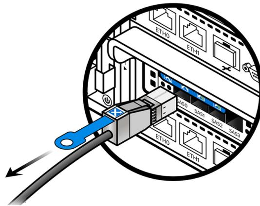
Figure 5-6. Removing a SAS Cable (Controller)
