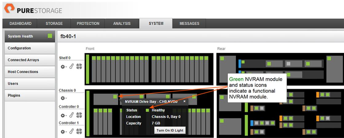
Figure 8-11. GUI Indication of a Functional NVRAM Module
